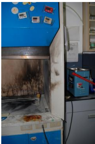
Mixing \text{KMnO}_4/\text{H}_2\text{SO}_4 /toluene causes fire
